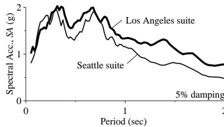
Figure 7. Median response spectra from earthquake suites. Each suite has 20 records.
